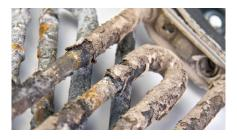
This image shows the heating element inside a boiler-based steam oven. As little as a 1/4" of scale buildup can decrease energy efficiency by nearly 40%. Imagine a typical combi oven that costs \$1,500 a year in electricity: a 30% reduction in efficiency, due to poor water quality, could mean up to \$450 in wasted electricity annually on one piece of equipment. Furthermore, it's not just the oven that may be increasing costs, but inefficiencies in coffee, espresso and ice equipment as well.
