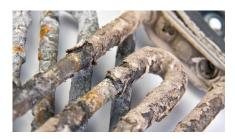
valves. Scale can cause valves and floats to stick, causing low water shutdown or leaks. Scale on the evaporator can cause ice to stick and refreeze with each cycle, causing "freeze up".
