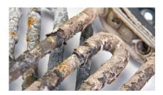
This image shows the heating element inside a boiler-based steam oven. As little as a 1/4" of scale buildup can decrease energy efficiency by nearly 40%. Imagine a typical combi oven that costs \$1,500 a year in electricity: a 40% reduction in efficiency could mean up to \$600 in wasted electricity annually, on one piece of equipment.
